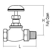
Glass-filled Teflon® disc is good for low pressure steam applications (150 WSP / 300 W), standard on all heavy
